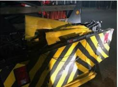
Left: An accordion-like attenuator on the back of our TMA normally looks like this, as it's designed to absorb the impact from a crash and protect crews up ahead. Right: A crash along I-5 on Oct. 30 smashed this attenuator flat.
