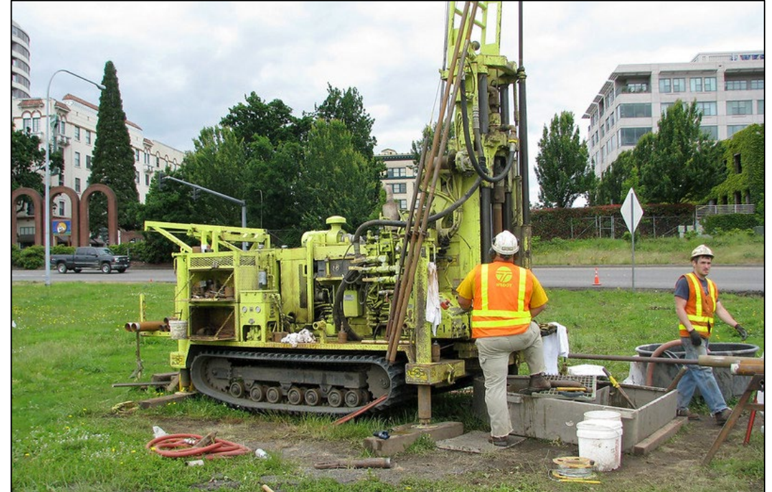
An example of the type of machines used for geotechnical drilling (Photo by WSDOT)
