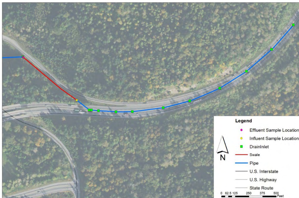
Figure 4. Mirrormont biofiltration swale monitoring site and associated drainage features
