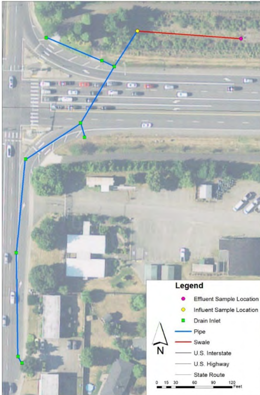
Figure 2. Vancouver biofiltration swale monitoring site and associated drainage features
