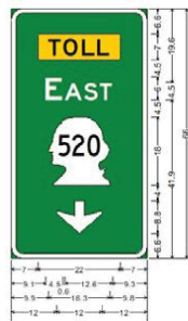
3.00' Radius, 1.25' Border, White on Green; "EAST", E 2K; M1-601; Table of letter and object lefts Letter E A S T Left 4.00 26.38 51.38 36.50 Right 13.00
