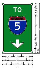
3.00' Radius, 1.25' Border, White on Green; "TO", E 2K; M1-41; Down Arrow Custom = 8.75" 270"; Table of letter and object lefts Letter T O Left 5.00 11.13 Right 5.00 15.13
